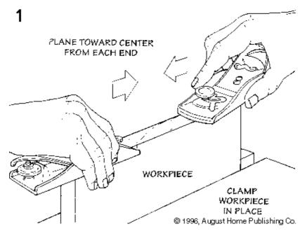
**PLANE TOWARD CENTER.** One simple method is to plane from either end toward the centre, see Fig. 1. This avoids the problem by not allowing the blade to catch on the unsupported ends of the work piece. The only problem with doing this is it can be difficult to plane a straight edge that's both smooth and flat.
