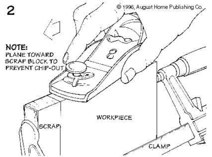
**ADD SUPPORT.** Here's a better solution. Clamp a scrap piece of wood to the end of the work piece, see Fig. 2.
